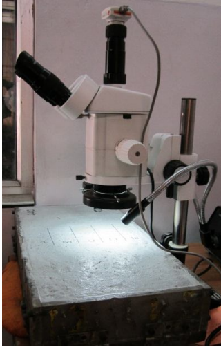
Fig. 4. Shrinkage crack measured in stereo microscope.
